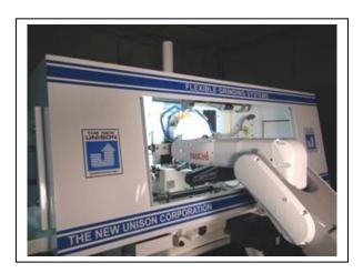
The Model 2150<sup>™</sup> utilizes Unison's proprietary software and control which allows your operator to customize centerless grinding, such as through feed, infeed & secondary operations, including plunge grinding, tapers and profile grinding of cylindrical parts with a range of diameters from 0.005" (.127mm) to 5" (127mm).
